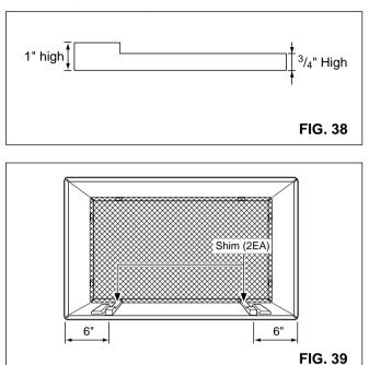
8 Install the new unit into the wall sleeve
